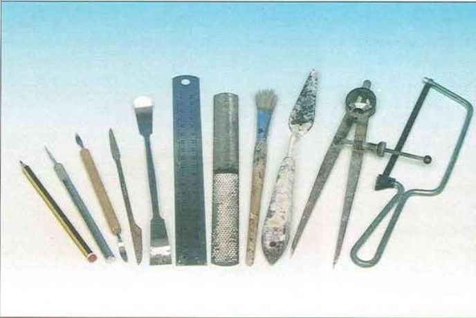
FROM LEFT TO RIGHT: PENCIL, MODELLING KNIFE, SCRAPER, ROUGH FILE, CLAW, RULER, RASP, BRUSH, TROWEL, COMPASS AND SAW.
